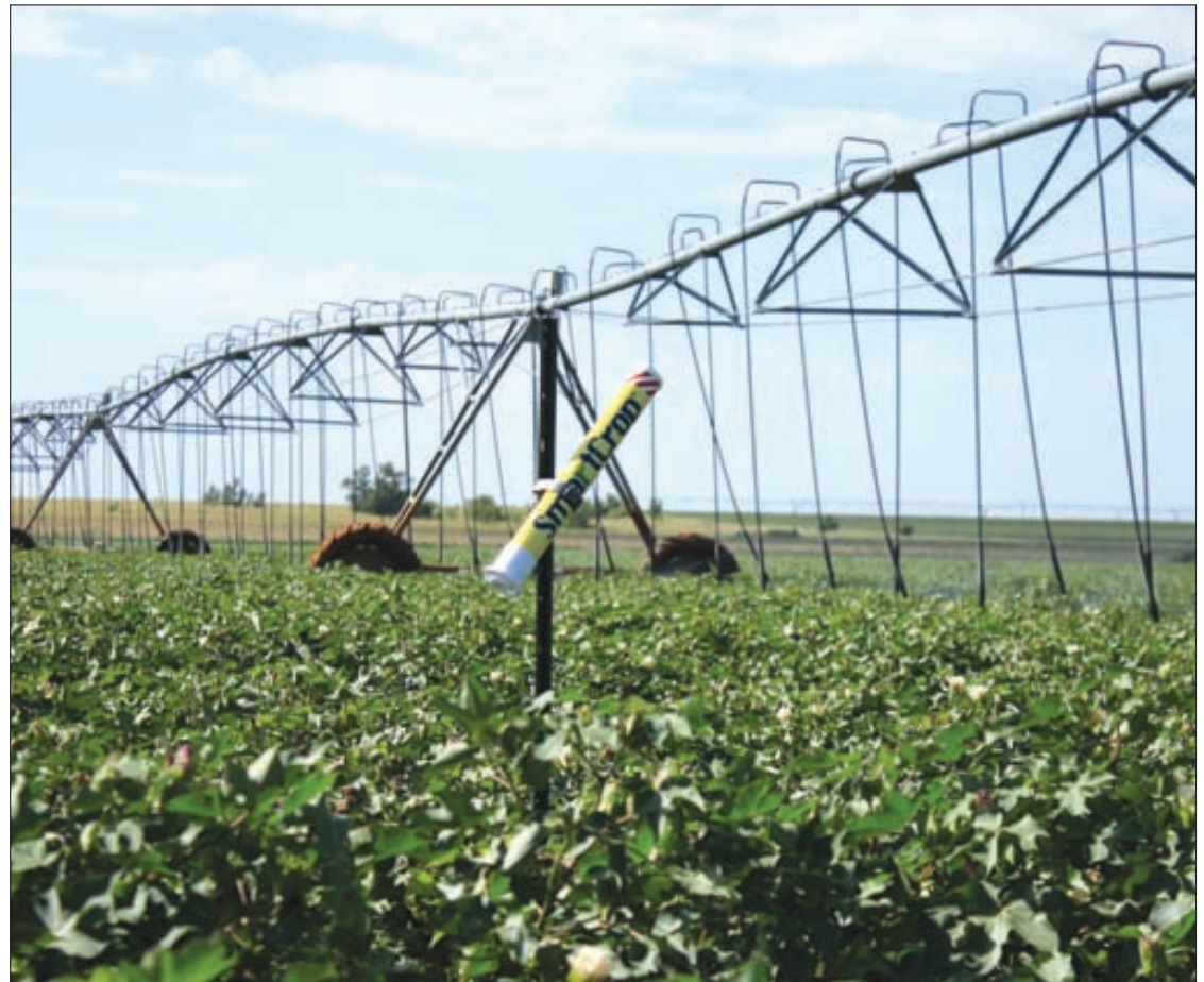
TOP TECH: Infrared sensors, which measure the crop canopy's temperature based on plant transpiration rates, make watering decisions easier. The technology is site-specific and does not rely on evapotranspiration readings, which can vary among fields.
